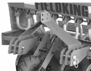
Fig. 14. Power transmission unit and its main components.
